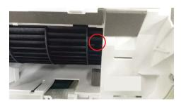
23) Hold and press the Cross Flow Fan to left side as much as possible, meanwhile, take Fan Motor out.
