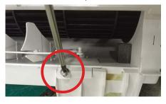
20) Remove the 2 screws of Louver Motor V to take the motor out.
