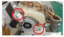
22) Remove 1 screw between Cross Flow Fan and Fan Motor.
