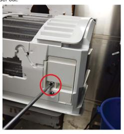
5) Loose the screw on Terminal Board and remove Unit-to-unit wiring.
