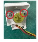
21) Remove 2 screw fixing the Fan Motor Cover, then remove Fan Motor Cover.
